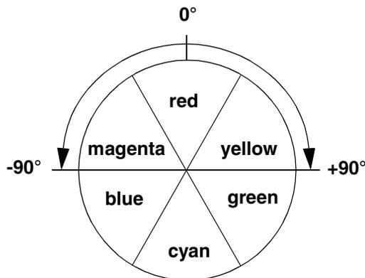
You set the hue adjustment using the **SetHue()** function. The **GetHue()** function returns the current hue adjustment. For NTSC video, you can adjust the hue from  $-90^\circ$  to  $+90^\circ$ . Because of the nature of PAL/SECAM signals, hue adjustments can't be made.
